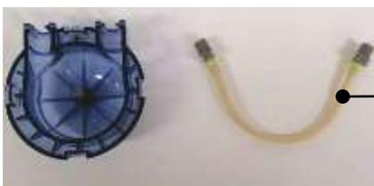
(7) Remove wash buffer pump tube.
