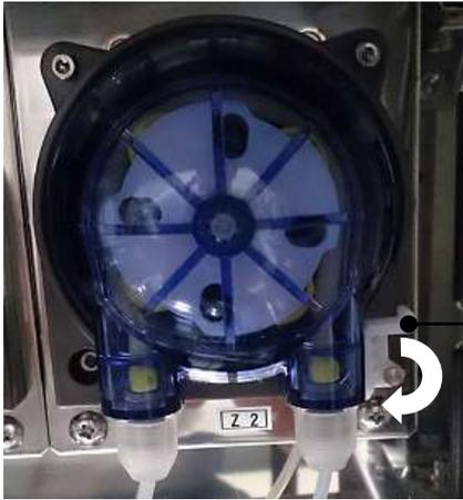
(3) Release wash buffer pump lock.
