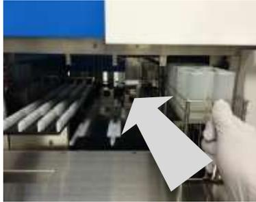
(4) Set wash buffer bottle in wash buffer bottle rack in drawer (at setting position No.4).
