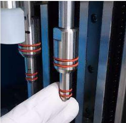
**(9) Fit new O-ring onto groove on dispenser.**
