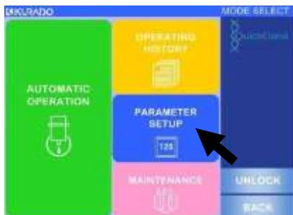
(1) Refer to "3.6 Start-up of System", turn system power ON, and move to mode selection screen.
