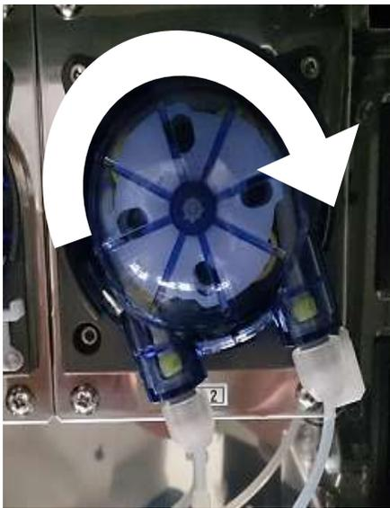
(11) Fit wash buffer pump in tilted position on fitting groove as shown in figure. Then turn wash buffer pump clockwise (in direction of arrow) until it stops (approximately 20 degrees).
