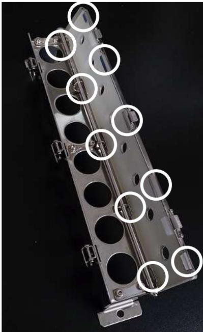
(5) Fit cleaned or new holder packing onto cartridge holder
