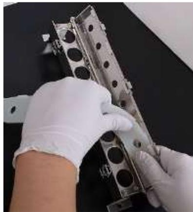
**Note:** If fitting of holder packing is omitted or incomplete, normal isolation operation may not be possible due to insufficient pressurizing. After fitting holder packing, be sure to confirm that packings are fit properly onto 10 cartridge holder hooks.
