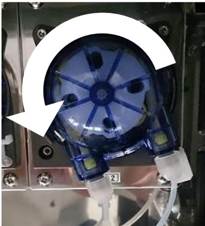
(4) Grasp plastic cover of wash buffer pump and turn counterclockwise (in direction of arrow) until it stops (approximately 20 degrees). Then pull and remove wash buffer pump toward you.
