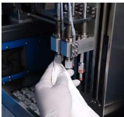
(8) Open sliding doors, refer to below and clean pressurizing nozzle (packing).
