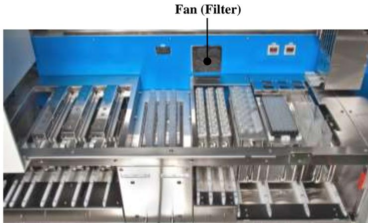
A fan filter is used in fan installed in rear of system work area. A fan filter is used inside the fan. Procedures for fan filter replacement are explained below.
