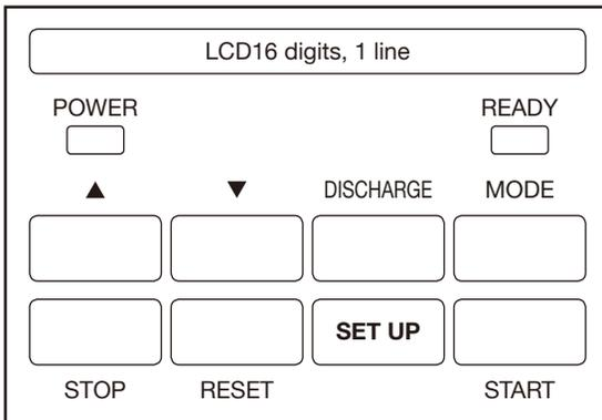
2. Press [MODE] button for necessary times to display the desired parameter.
