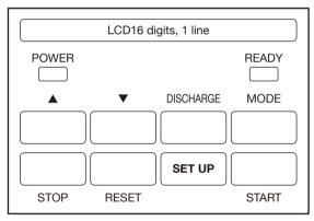
2. Press [MODE] button for necessary times to display the desired parameter. [DISCHARGE] button is pressed to return to the previous parameter. After the last parameter, the display returns to the first parameter.
