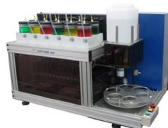
Weighing multiple dyestuffs simultaneously by using a dispenser. Mini volume measurement type with a turntable.
