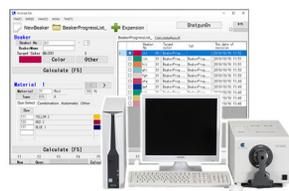
Measuring the target colors, and making a recipe with selected dyestuffs or requested combination of dyestuffs.
